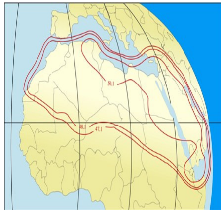
fig.2 EIRP contour map for NILESAT 101 satellite
