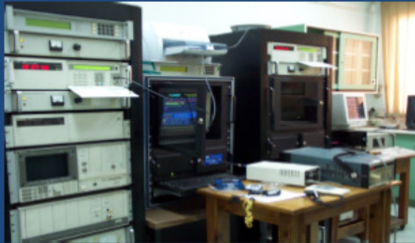
Controlled Cesium Clock and the International Frequency Traceability System with Accuracy of 5 \times 10^{-13}
